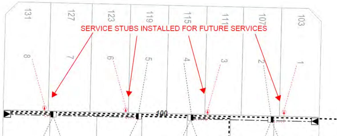
**Figure 5-5: Rear Lot with No Lane – Pedestal Layout for Staggered Lots**
