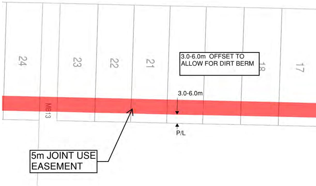
**Figure 5-14: Easement Offset for Developer Berm (Example Only)**
