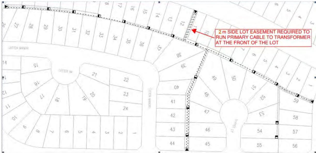
**Figure 5-3: Rear Lot with No Lane – Side Lot Easement Example 2**
