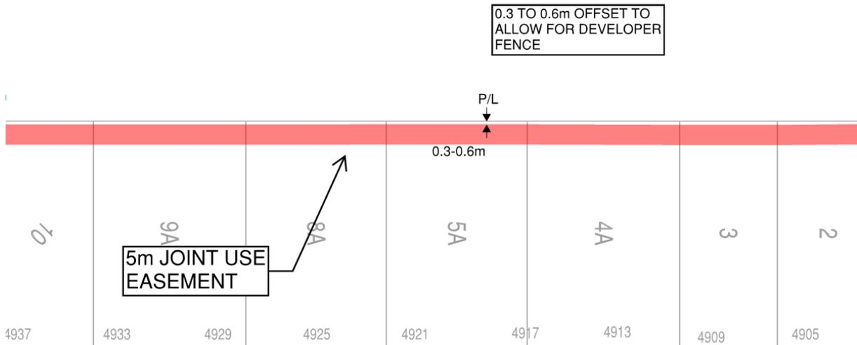
**Figure 5-13: Easement Offset for Developer Fence (Example Only)**
