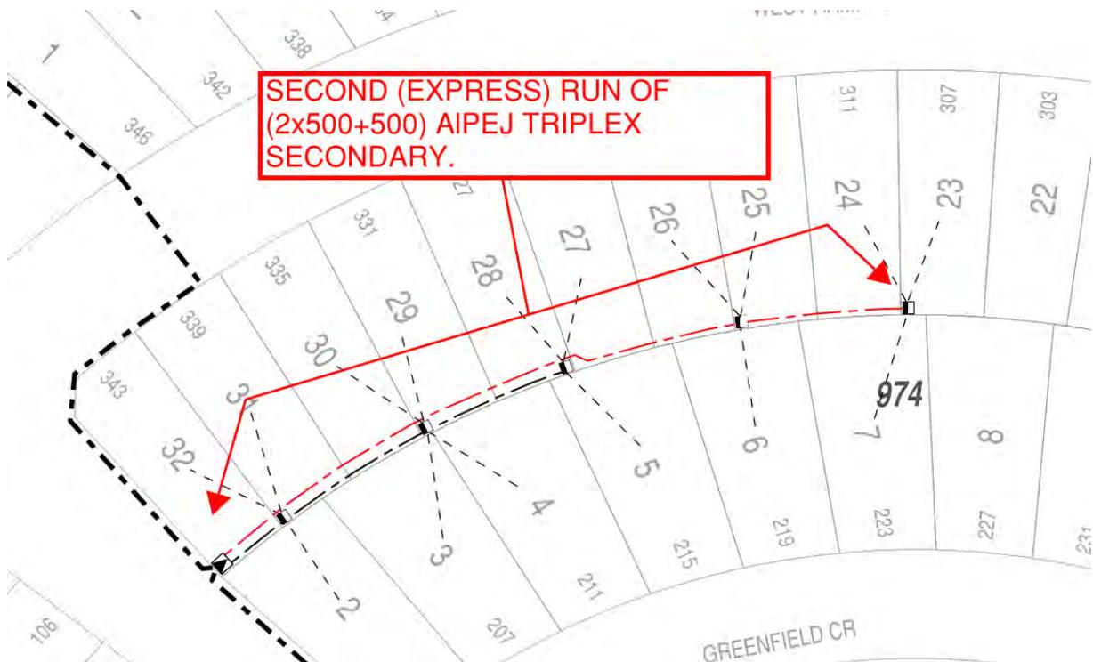
**Figure 5-1: Rear Lot with No Lane – Transformer Layout**
